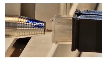
• Inconsistencies and Flashing from Molding: Another significant challenge was dealing with inconsistencies in the parts due to flashing from the molding process. Engineering a solution involved developing adaptive algorithms within the machine's control system to detect and compensate for these variances, ensuring consistent part handling.
